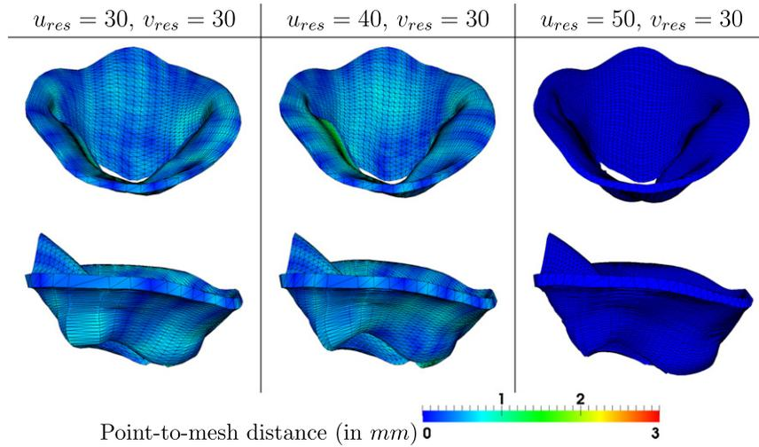
Fig. 10. Effect of the circumferential resolution  $u_{res}$  on the simulation. Only millimetric differences were visible. Colors encode point-to-mesh distance computed with respect to the solution obtained at  $u_{res} = 50, v_{res} = 30$ . (For interpretation of the references to colour in this figure legend, the reader is referred to the web version of this article.)
