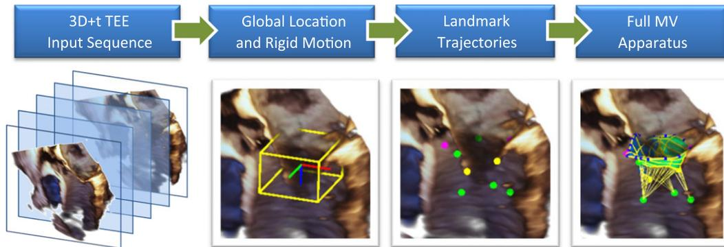
Fig. 4. The main steps of the automatic estimation pipeline. We first estimate the global position of the MV, then detect the MV landmarks inside this region of interest and finally map and deform triangulated surfaces to segment the MV leaflets.
