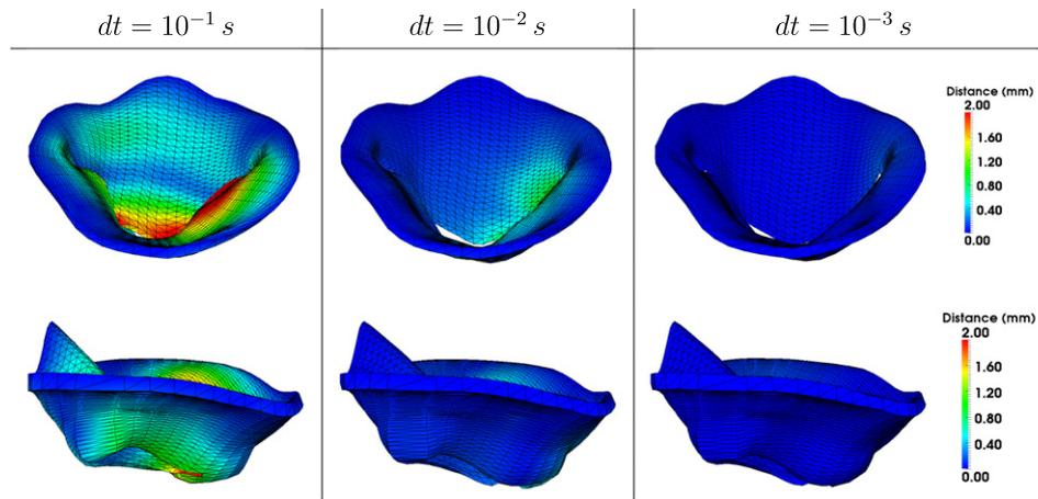
**Fig. 12.** Effect of the time step  $dt$  on the simulation. Colors encode point-to-point distance computed with the result obtained at  $dt = 10^{-4}$  s. Convergence was achieved at  $dt = 10^{-3}$  s but  $dt = 10^{-2}$  s already yielded voxel accuracy. (For interpretation of the references to colour in this figure legend, the reader is referred to the web version of this article.)
