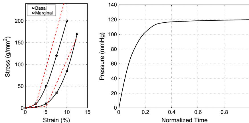
**Fig. 7.** Left panel: Stress–strain behavior of chordae. Linear approximation in dashed lines (data from Kunzelman and Cochran (1990)). Right panel: Pressure profile applied to the leaflets to simulate closure. The time is adjusted for each patient to match valve closure duration.
