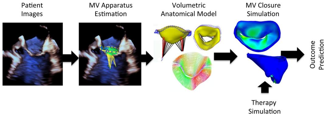
Fig. 2. The main steps of the proposed framework for MV closure simulation.
