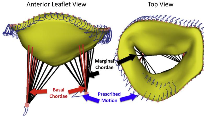
**Fig. 6.** Tendineae chordae and boundary conditions (Patient 25). Chordae are inserted in the leaflets at the same spatial location for all patients owing to the point correspondence. Mitral annulus and papillary tips motions are prescribed from image data.
