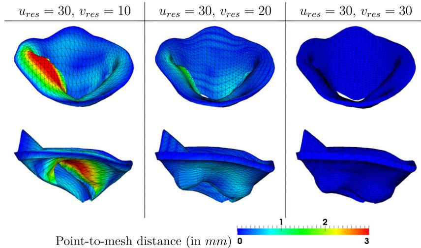
Fig. 11. Effect of the radial resolution  $v_{res}$  on the simulation. At  $v_{res} = 10$ , MV closure simulation yielded a totally different result (see posterior leaflet), while convergence can be seen for  $v_{res} \geq 20$ .
