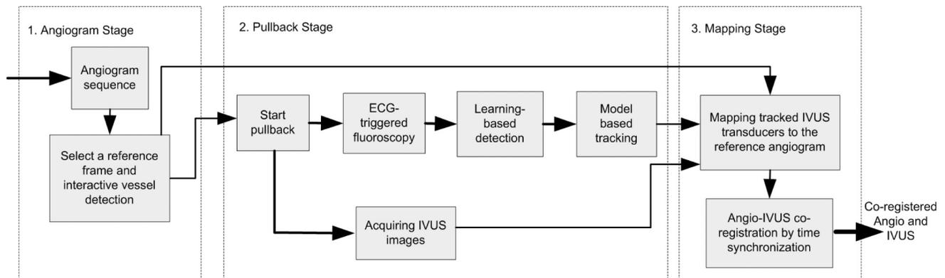
Fig. 3. Co-registration system workflow.
