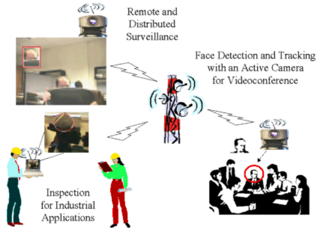
Figure 1: Intelligent processing and summarization of video in a radial network of cameras. Wireless connections can be employed for the transmission of data of interest to the central processing unit.
